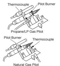
Figure 39 - Correct Pilot Flame Pattern
